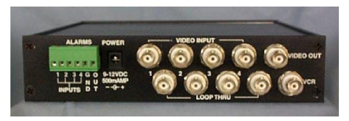
LEDs on the front of the QS-402HR. The green one to the far left will be illuminated continuously when power is applied. Next connect the four BNC video inputs to the unit from the cameras or video sources. As seen above they are labelled 1-4 corresponding to the four front panel buttons. The two BNCs to the left are the video outputs and should be connected to the video monitor. If connected directly to the video monitor and no other looping devices then this monitor should
